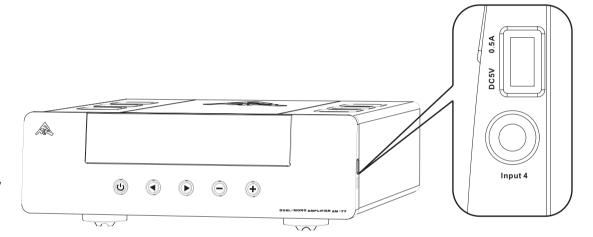
When the 3.5mm jack is used, disconnect the RCA connecion to Input 4 at the rear of the AM-77
